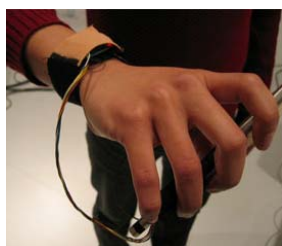
Figure 2. Wireless module and sensor.
