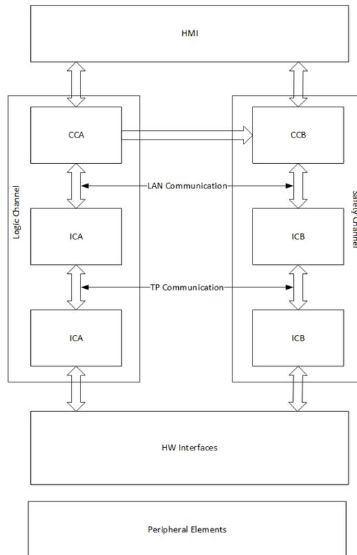
In opposition to the two-channel architecture of the above cited Communication Controller (CC) the HMI contains only one software channel. The safety relevant information items – display information or operator commands – are handled according special methods providing the safety via two-fold and threefold communication with the safe central layer and acknowledgment of each step by the user so that SIL4 is reached. This concept is called the method safe HMI.
