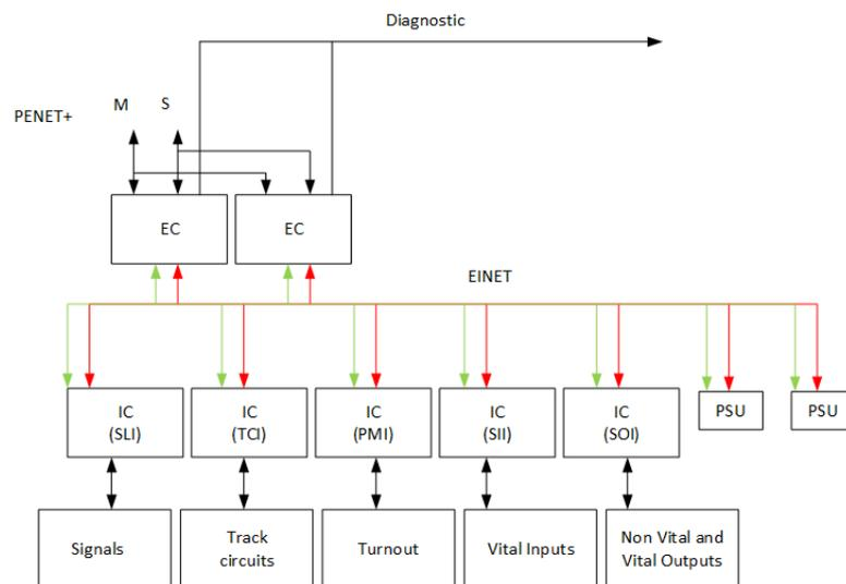
EC are processor units that arrange vital communication between functional core layer units on the one side and units IC on the second side.
