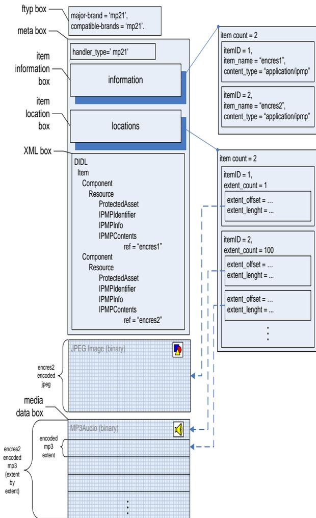
**Figure 2 – Simple protection (only digital resources)**
