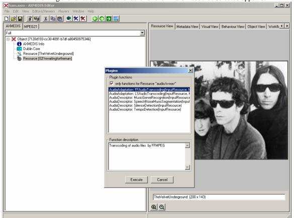
The first audio adaptation function available is the FFmpeg transcoding function which is selected by clicking on **FFAudioAdaptation: FFAudioTranscoding**. A new window appears showing the interface to the audio transcoding function. In the example of the following figure, the transcoding function is used to create a 10 second snapshot with reduced bit rate of the input audio file:
