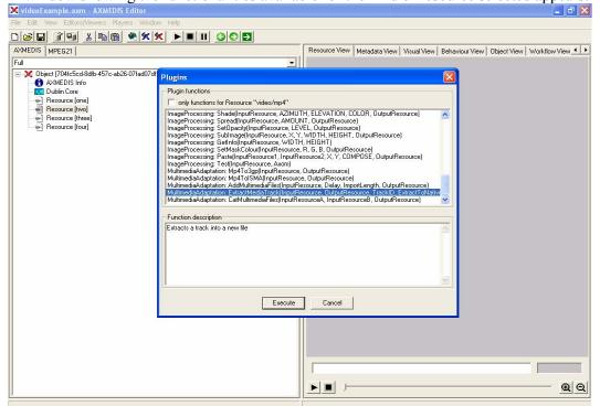
The ExtractMediaTrack function allows extracting a media track from an input MP4 resource into a new resource. In this example, we extract the first track of the input resource. The first track is an audio track in MP3 format. The extraction is selected to be in non-native format i.e. the extracted media track will not be a MP3 file but it will be converted to MP4. Once extracted, further adaptation can be performed with other plug-ins.
