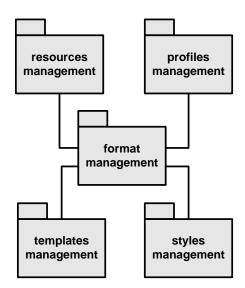
Resources and profiles (user, device and context profiles) represent the input to the Format Engine; selected templates and styles are its output and they are used to create the SMIL presentation; the format management implements the filtering and optimization logic.
