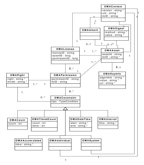
Figure - OMA DRM REL UML Class Diagram
