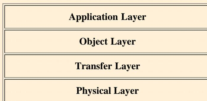
**The Intel 82527 chip was chosen for our CAN module and it will realize the physical, transfer and object layer of this structure. The CAN system it is based on a packetized communication, there was four frame type:**
