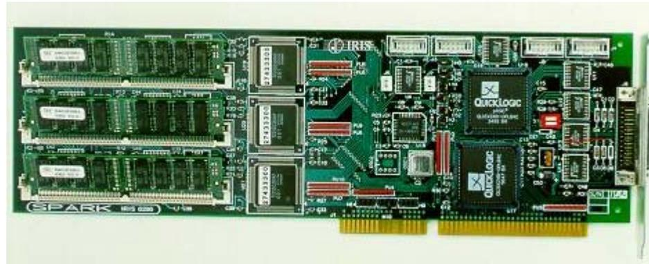
The SPARK system is based on a synchronous multiprocessor architecture using IRIS custom-designed digital signal processing units. Each DSP board is based on three custom DSPs connected in a synchronous configuration and operating in parallel at full speed. The total aggregate computing power is 150 MIPS (peak) per board, and on-board interconnection bandwidth reaches 26 Mbit/s.
