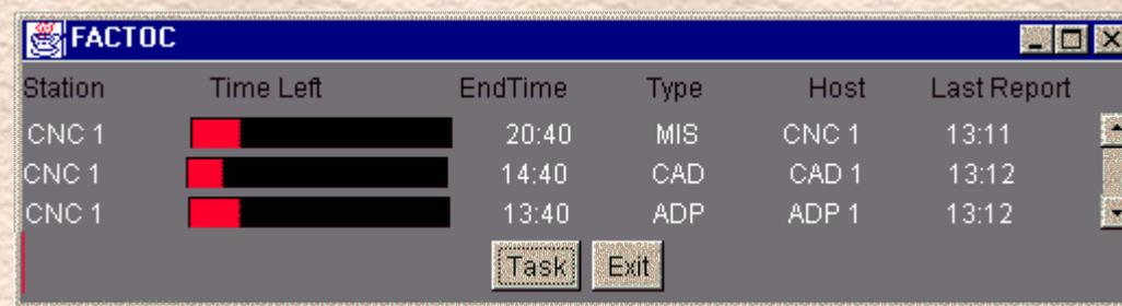
The FACTO Client Optimizer shows to the operator all the operation to be performed on the CNC that he controls.
