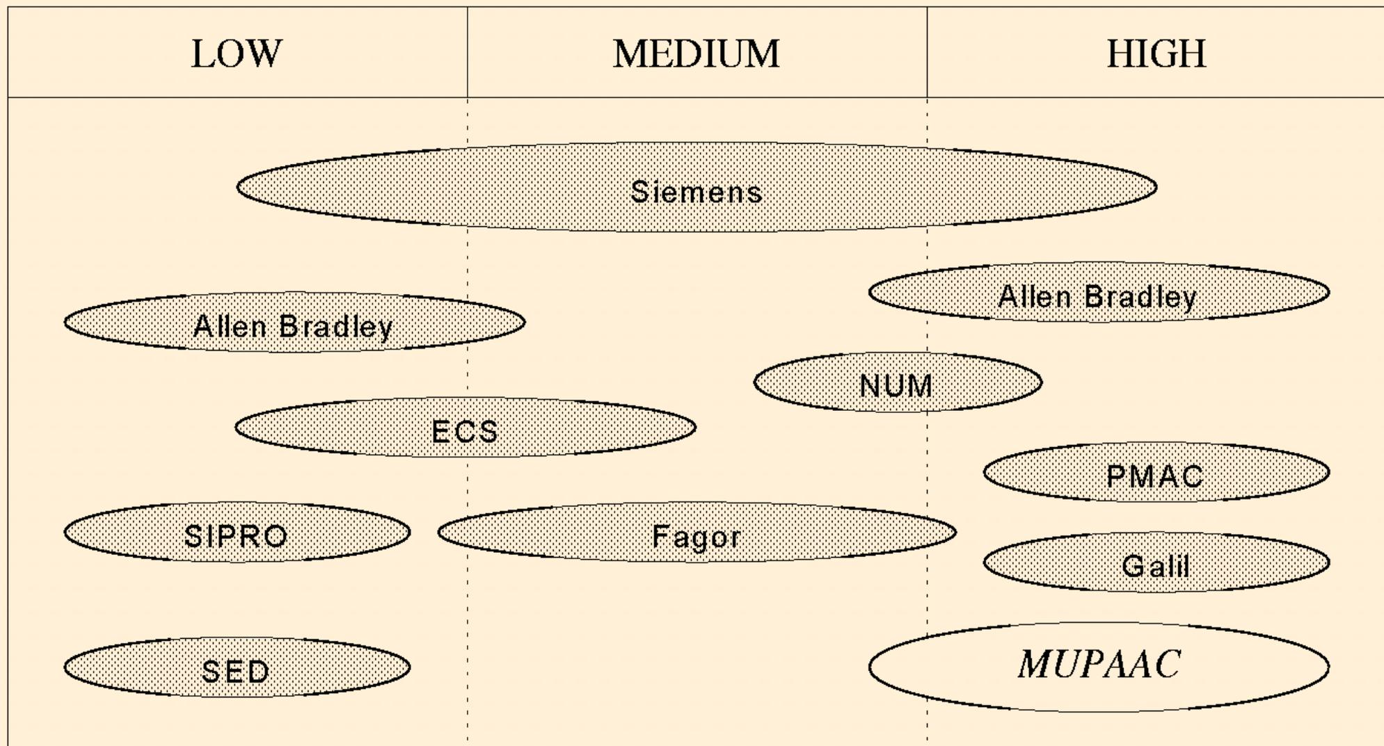
Please note that some firms present several types of solutions which are capable of covering different sectors or the market -- e.g., Siemens, ECS, etc. Presently the controllers which are employed on cutting, soldering, moving, machine tools belong typically to MEDIUM and LOW categories. The adoption of high performance will improve the precision of elaboration allowing the adoption of more complex tools such as lasers, elaborations directly at the final resolution on milling machines, etc.
