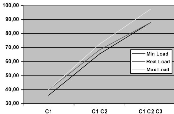
The figure reports the load of the network. In order to measure the effective performance, three couple of machines have been tested separately so to evaluate the maximum load on the HUB. The HUB has been guaranteed to have at least 90% efficiency under any workload conditions. C1, C2, C3: the three couples versus the load shown in Mbps.
