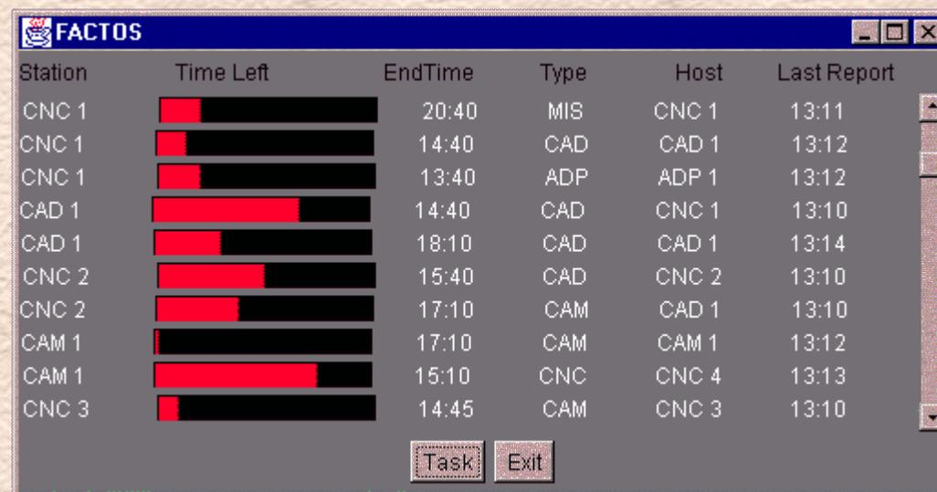
The FACTO Server shows to the manager all the work (and their status in real time) for all the CNCs and CAD/CAM/Adaption stations in the factory.
