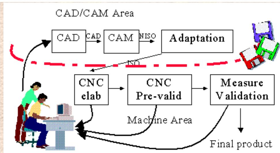
In the industries producing templates, there exists a strong interest in the integration of CAD/CAM with the factory part in which MMs, measurement systems, robots, etc., are present. The integration must be supported by a fast and reliable communication between these two areas for making available
