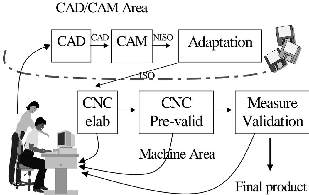
In the industries producing templates, there exists a strong interest in the integration of CAD/CAM with the factory part in which MMs, measurement systems, robots, etc., are present. The integration must be supported by a fast and reliable communication between these two areas for making available
