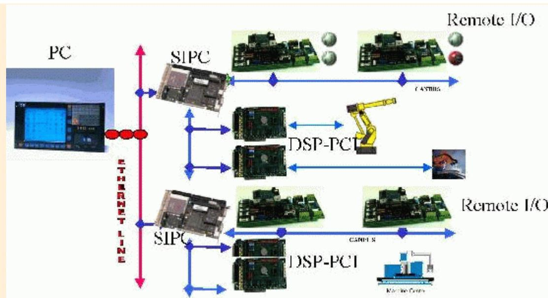
MUPAAC activity plans to adapt the INDEX-DSP architecture of SED. In particular, this action will consist in improving INDEX-DSP performance and functionalities by using HPCN technologies: removing the LOGIPACK, RS232, RS 485 and the dual port memory communication supports and substituting them with the more efficient mechanisms such as CANBUS and PCI protocols. The adaptation of INDEX-DSP will be an efficient support for focussing this project on technology transfer. For these reasons:
