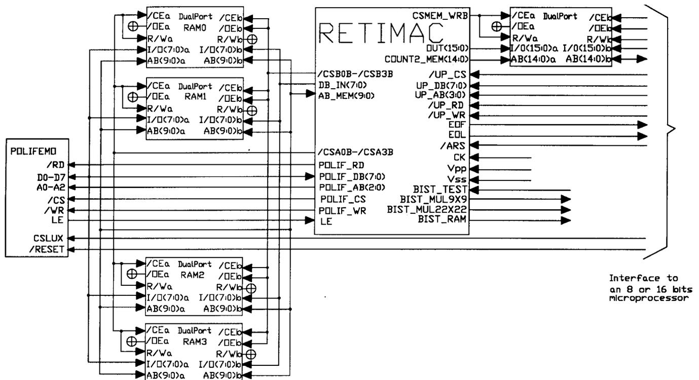
Fig. 4. Architecture of a system based on RETIMAC grabbing the images with the Polifemo chip.
