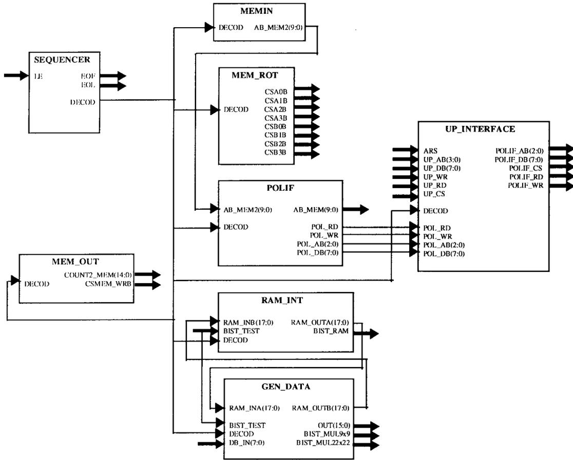
Fig. 5. RETIMAC block diagram.
