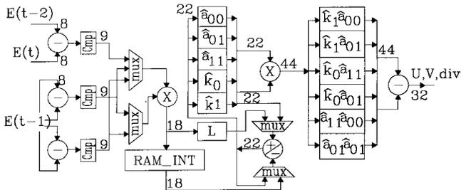
Fig. 6. The main blocks of RETIMAC data path.
