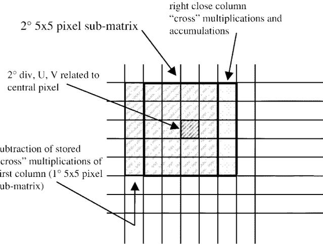
Fig. 7. Technique for estimating the next velocity vector by using read-modify-write operation of internal RAM.
