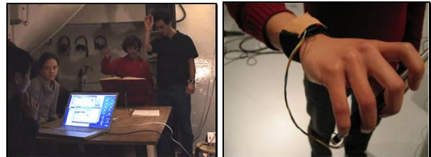
Figure 6. The Score Follower listens to the player and provides automated “page turning” and accompaniment.
