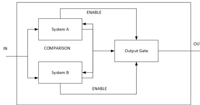
Fault detection may be incorporated in each system through monitoring the outputs of other sets of equipment. Voting is generally based on a simple majority with the facilities to shut down any equipment out of step.
