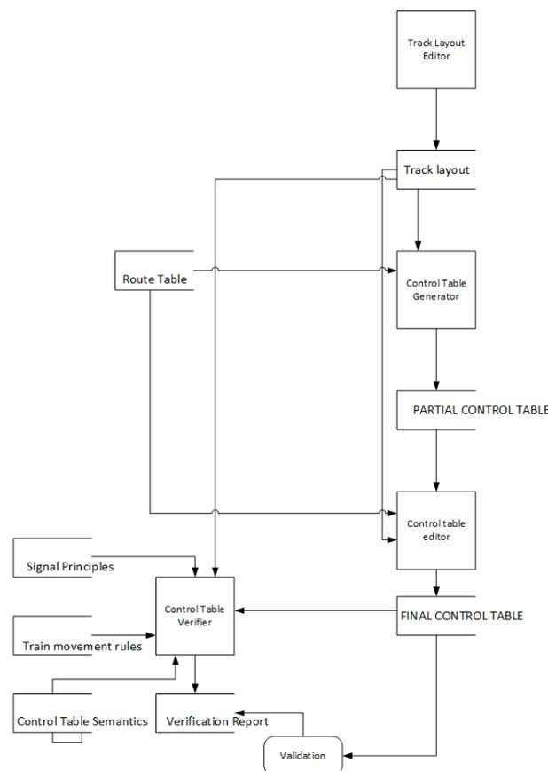
In the figure above it is showed the process flow of generating the control table. It is possible to identify 4 main processing units:
