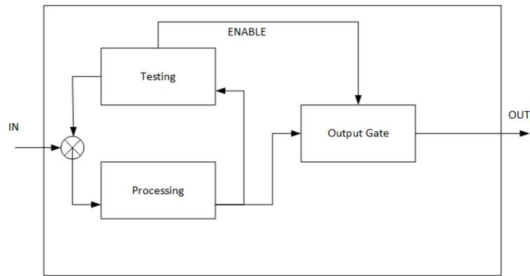
The fail-safe system will not generate provocative outputs under fault conditions and outputs will be inhibited should incorrect outputs be detected by processing of the test function. Some consideration of single channel systems is:
