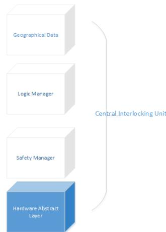
The processor could be based on CPUs or PLC (depends by the type of the interlocking) and a redundant management unit.
