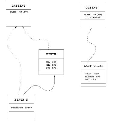
Figure 3: Relationships among classes: is-a as continuous lines, is-part-of as dashed lines, is-referred-by as dotted lines.
