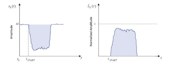
Figure 2. Example of extracted information,  $\hat{s}_k(t)$ , for a generic received signal  $s_k(t)$ ;  $t_{START}$  indicates the instant when the entrance door opens.
