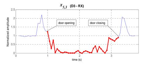
Figure 4. An example of the useful signal portions used in the next stages processing is highlighted in red (please note that this signal has been taken before calibration as in Figure 2 left).
