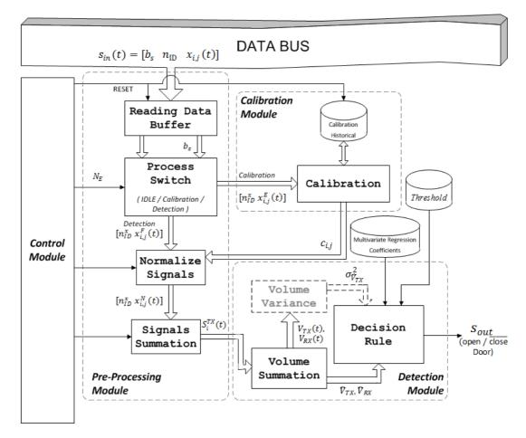
Figure 7. Block architecture of system real-time implementation.
