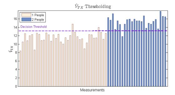
Figure 6. Threshold for  $\hat{V}_{TX}$  over a mixed set of test measurement (one and two people) accessing the inner cabin.
