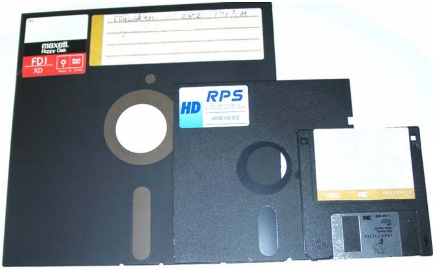
The image shows three floppy disks of different sizes. On the left is a large 8-inch floppy disk with a white label that includes the Maxell logo and 'FDI XD'. In the middle is a 5.25-inch floppy disk with a blue label that says 'HD RPS'. On the right is a smaller 3.5-inch floppy disk with a white label. The disks are arranged in a slightly overlapping manner against a light blue background.
