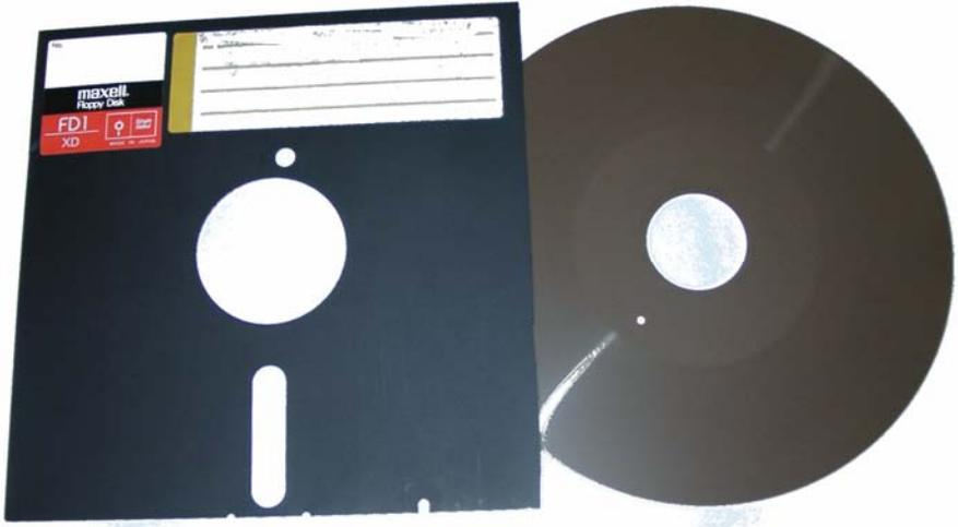
The image shows two floppy disks. On the left is a 5.25-inch Maxell FDI XD disk with a white label. On the right is an 8-inch floppy disk, which is significantly larger and has a dark surface with a central hole.
