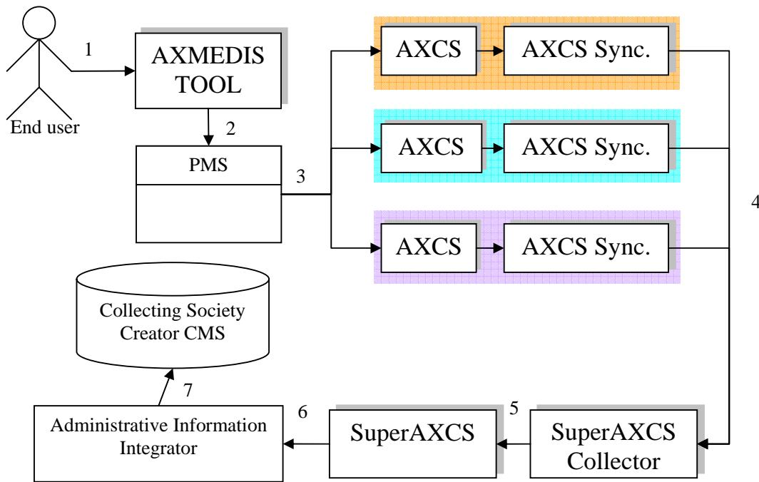
1. End User uses an AXMEDIS tool to operate on an AXMEDIS Protected Objects that are on different distribution channels
