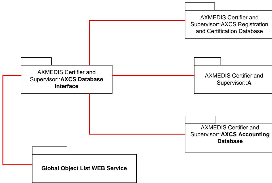
The Global Object List Web Service is a web application running on a web server implemented as a set of scripts. It has to provide to the system the possibility of retrieving information about all the objects present in the system. Given some data (typically a set of metadata) a requestor has to be able to recover all references about objects that are compliant with the given data.
