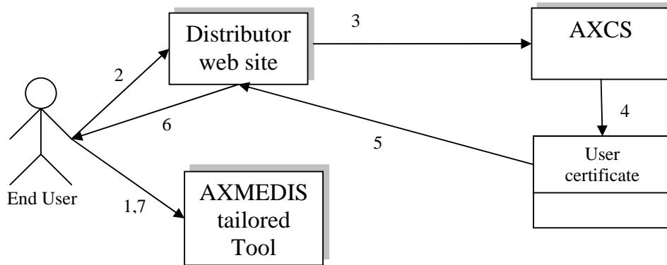
1. Upon first use the AXMEDIS tool (tailored by a distributor) checks for an user certificate. Assuming no certificate is found, the tool opens a web browser connecting to the web site of a distributor supporting registration of new users;
