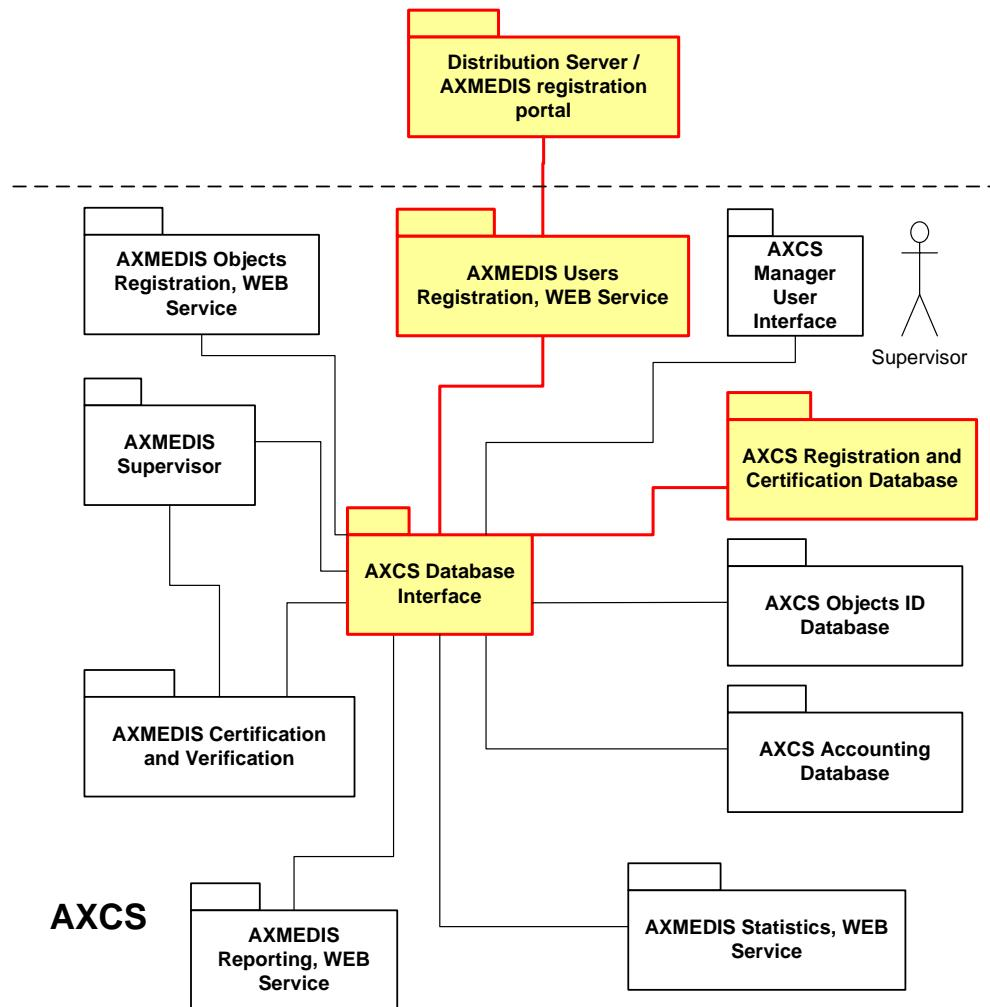
It can be identified the following logical decomposition in the structure of the User Registration Web Service:
