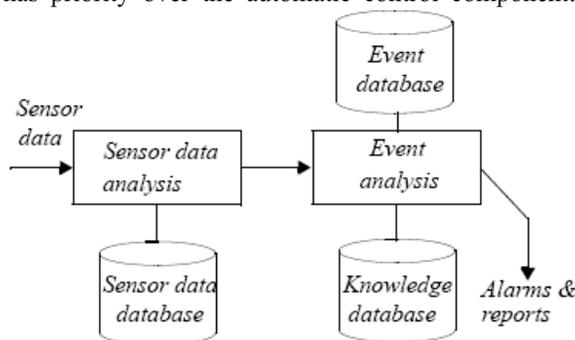
Figure 2. The sensor data analysis module followed by the event analysis module.
