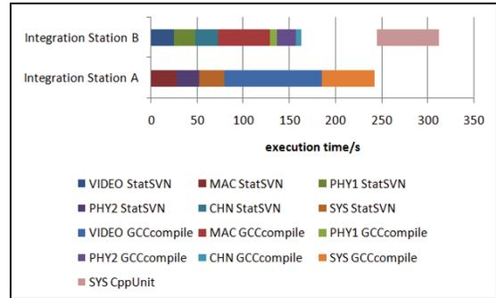
Figure 7: A worse case of job allocation with two Integration Stations
