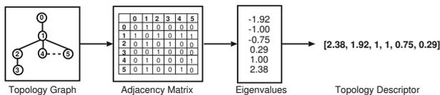
**Figure 4. Block diagram for topology descriptor computation.**
