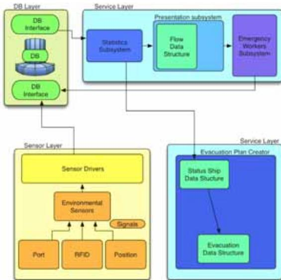
Figure 2. The emergency management system architecture
