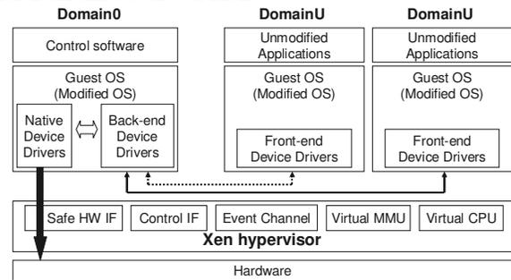
Fig. 2 The architecture of Xen with 2 DomainUs [8]
