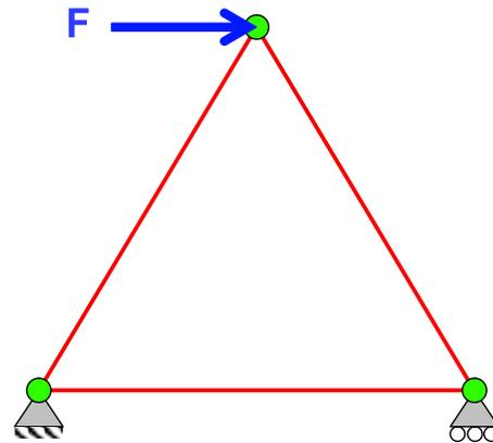
Figure 1. Example of a statically-determinate truss.
