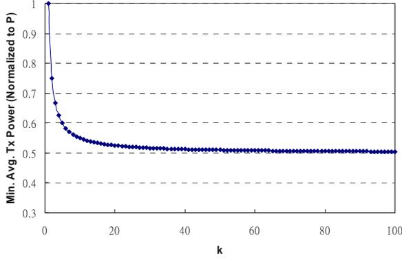
Fig. 3: Minimized average transmission power
