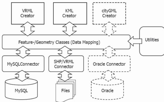
Figure 2: CAT3D Service Framework architecture
