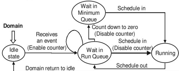
Fig. 8 State diagram of Upper-Bound design
