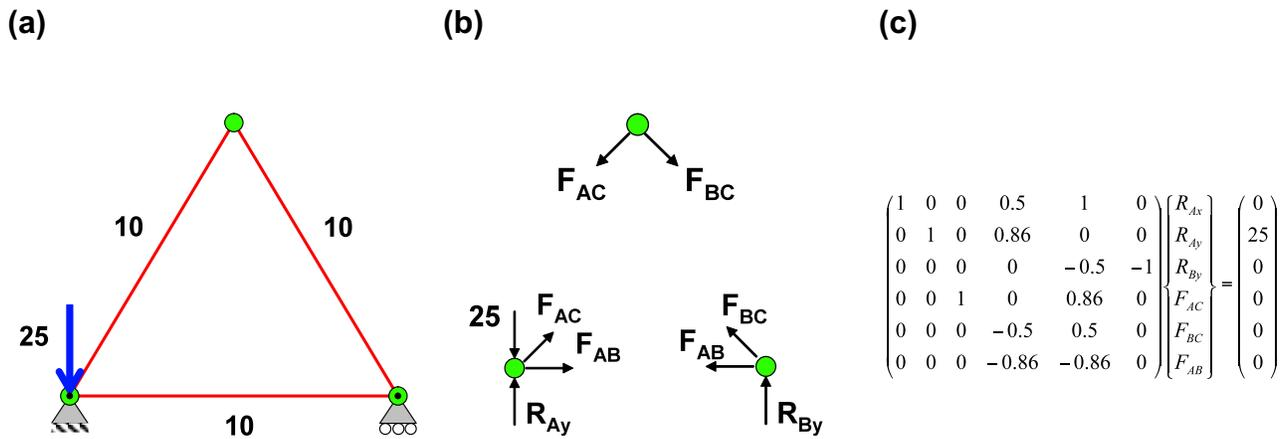
Figure 4. Sub-layer illustrations from the sketched-truss analysis layer: (a) valuing of recognized truss elements, (b) assembly of static equilibrium equations into a matrix format, and (c) solving of assembled static equilibrium equations.
