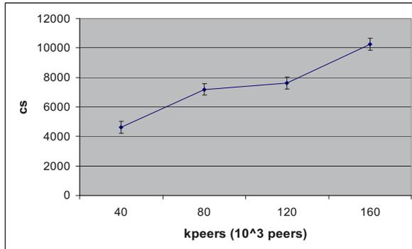
**Fig. 2 – AXTrack context switches per second**
