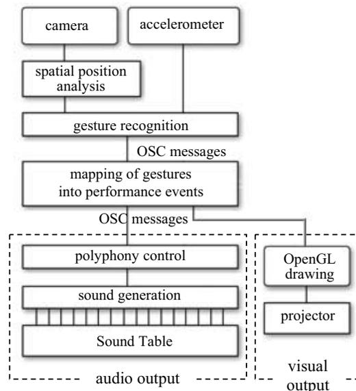
Figure 4. System processing flow
