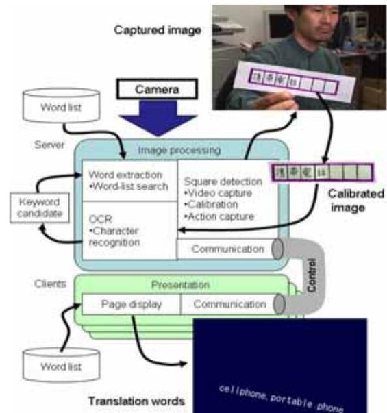
Figure 4: System architecture
