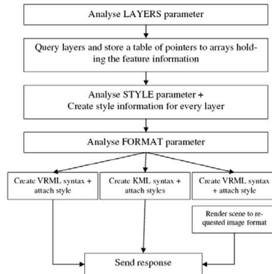
**Figure 1:** W3DS GetScene request example and the process of creating the response within the CAT3D framework (simplified).
