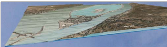
Figure 20. Simulation of the flood of the Loire river (France) showing part of the Town of Blois becoming an island. Different water levels on different areas can be moved up and down.
