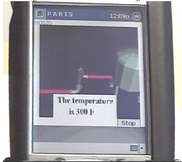
Figure 7: The pipes are highlighted in red, and a label is displayed as a result of a speech-driven query for the temperature in the pipes.
