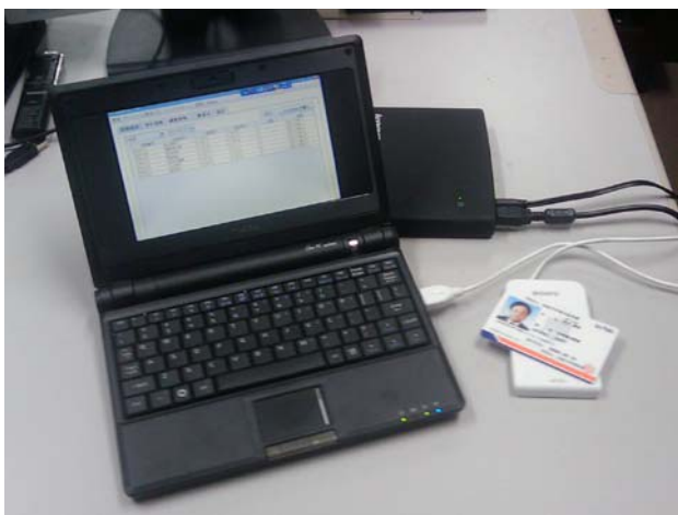
Fig. 4: The attendance management software and Pasori IC card reader
