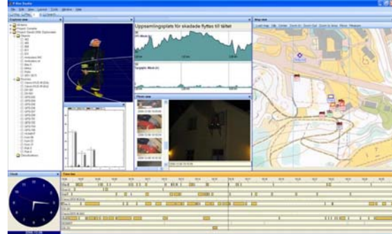
Figure 3. Synchronized visualization of sampled data and multimedia information for contextual analysis in F-REX Studio. The current layout displays a priori information, timeline, photos, video, a map with GPS tracks, heart rate, altitude, stance and statistical metrics.
