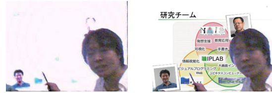
Figure 10. Left: a color image whose background is subtracted using AIR keying (Extracted Image). Right: the result shown on SyncSurface Board, which is the color image synthesized with the digital content.
