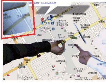
Figure 8. Digital contents and physical contents are projected onto the users' hands (center) and onto the notebook (upper-left) that a user holds in his hand.
