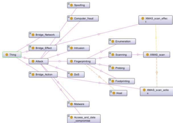
Figure 3 An example of the ontology of attacks in the case of the x-mas scan intrusion
