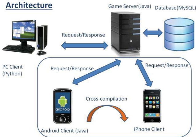
Figure 9. DeBugger Architect including Mobile Debugger. This shows the relationship between a PC Client, Android Client, iPhone Client and the Server
