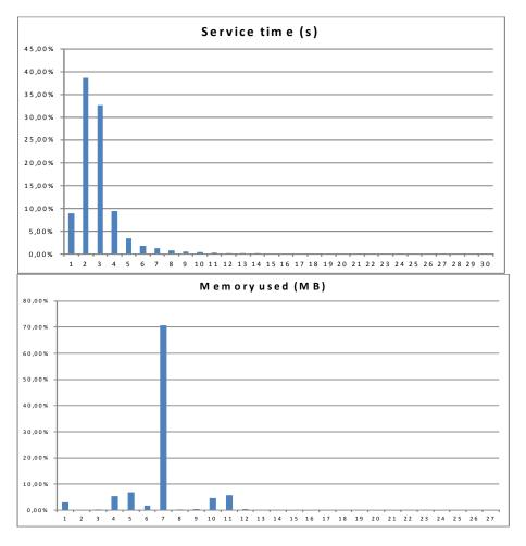
It can be seen that 93.21% of the requests were performed in less than 5 seconds and that 99.03% of the request were performed with less than 11MB.
