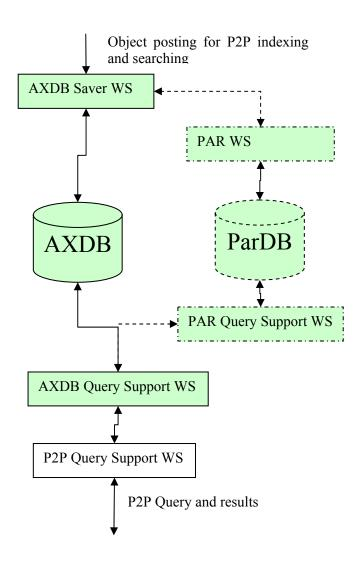
The posting of an object to the AXDB is done by the submission of a simplified object without the resources since it is only necessary to index metadata of the object and not to store the entire object in the AXDB. Moreover it is possible to save also bittorrent information by adding a custom metadata field that can be recovered by using the query mechanism together with the AXOID.
