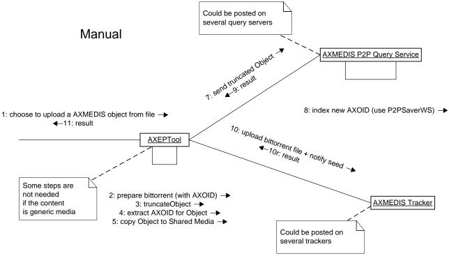
In the manual version some content manipulations which has been performed by AXCP, has to be done by AXEPTool, the AXOID has to be extracted for augmenting bittorrent, and the AXMT file (truncated object) has to be posted for future queries.
