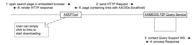
The first diagram shows the interaction between AXEPTool and AXMEDIS P2P Query Service. The action is simply to redirect the user query to the Query Service collecting in the response information regarding the matching objects. The WS response is processed, since all the present metadata have to be attached to the query result items.
