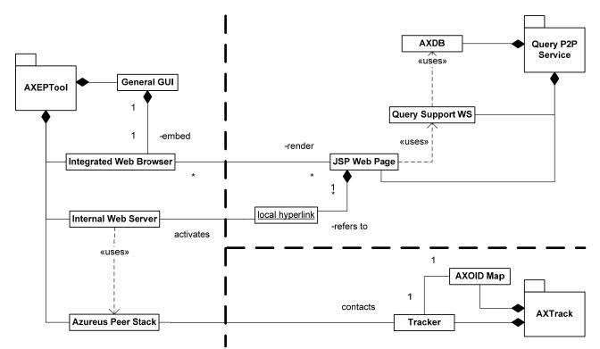
All modules are quite simple in terms of interaction. As most of Web Services implemented in Milestone 1 and 2 are REST web services, the JSP is the main entry point of the communication between server and the client. The integrated web server also serves as a user interface. Then the tracker communicates with the usual peer to peer stack.
