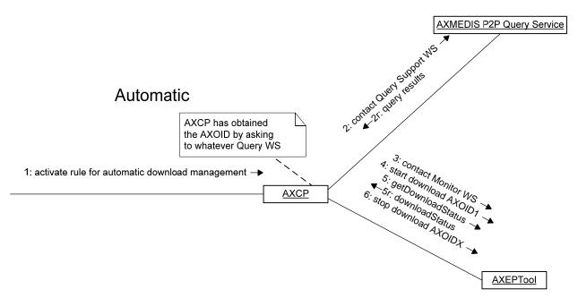
In the last diagram the AXCP is put as an intermediate in the AXEPTool control. In this case it allows the script function to operate as the user on the GUI (i.e. looking what is downloading and controlling those processes).
