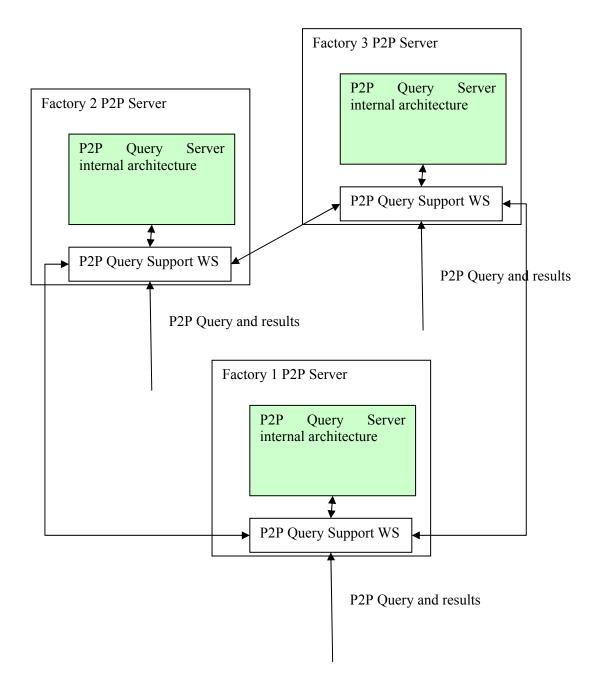
In this model the query on each factory can propagate to aumatically to other facories and the results are collected togheter by the P2P Query Support WS layer of each factory that became then a complex component replicating the functions of the MainQuerySupport at the P2P level.
