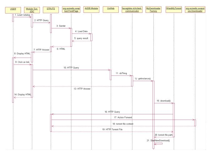
This involves most parts of the software, so it's a good introduction to the general architecture of the whole Axmedis P2P infrastructure. In this scenario, the user first browses the catalog of available media files from the FrontPage servlet (which gets it from AxDB). The result is then displayed in the integrated web browser.
