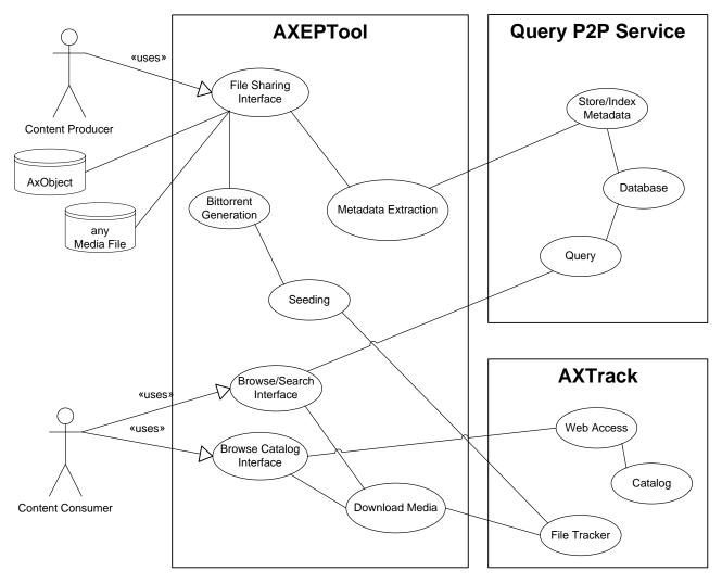
The content producer connects to a file sharing interface and use it to put the file on the peer to peer network. First metadata and bittorrent info are generated locally from the file. Those metadata are then uploaded to one or more AXMEDIS P2P Query Service, where they are indexed for subsequent query, and to one or more AXTrack Web Service as seed notification. The File Tracker starts keeping track of the files.
