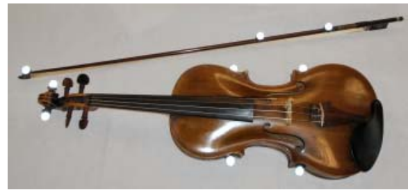
Figure 4. A violin and bow with markers for 3D motion capture.
