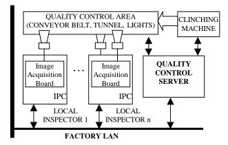
Figure 1. VISICON Hardware Architecture
