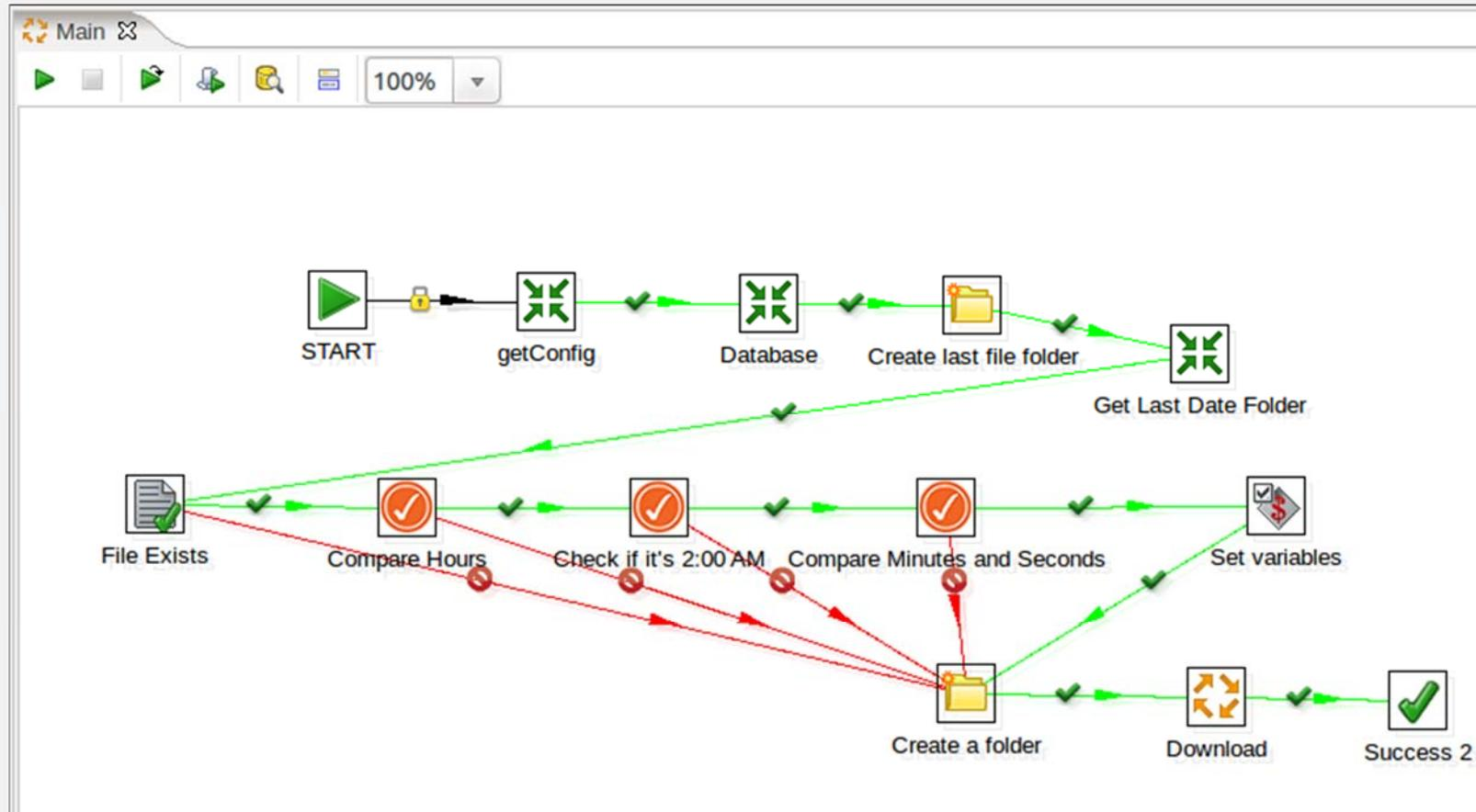
This Job is the same seen before for ingestion. The only difference is that it checks if there are two different datasets at the same hour.
