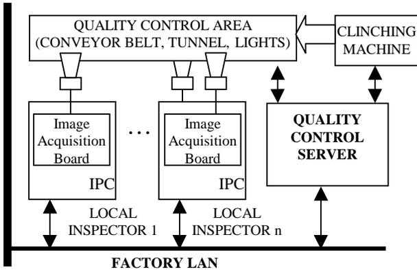
Figure 1. VISICON Hardware Architecture
