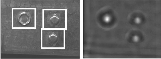
**Figure 4a. A good and two defected buttons with Target image segments.**
