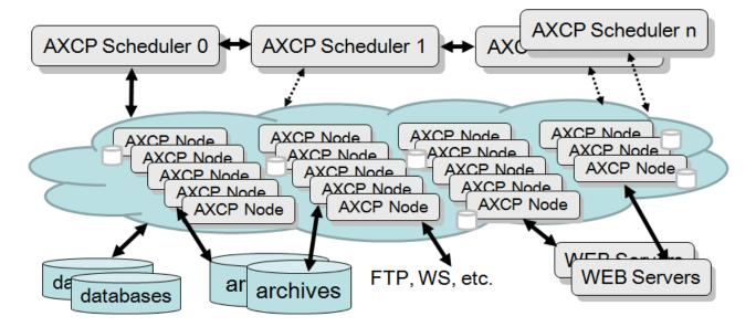
AXCP solution may be set up on a single computer with all inside as well as on many industrial or desktop computers (that may put at disposal a part of their CPU power and file system). Each node may share file systems and access independently on the network and thus on databases. Thus, solutions with large numbers of distributed databases are possible; to realize data and/or computational GRID solutions with shared or partitioned databases and data sources.
