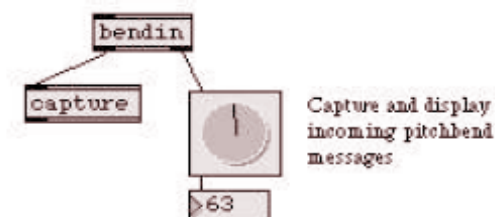
Figure 18: A simple program written graphically using MAX/MSP
