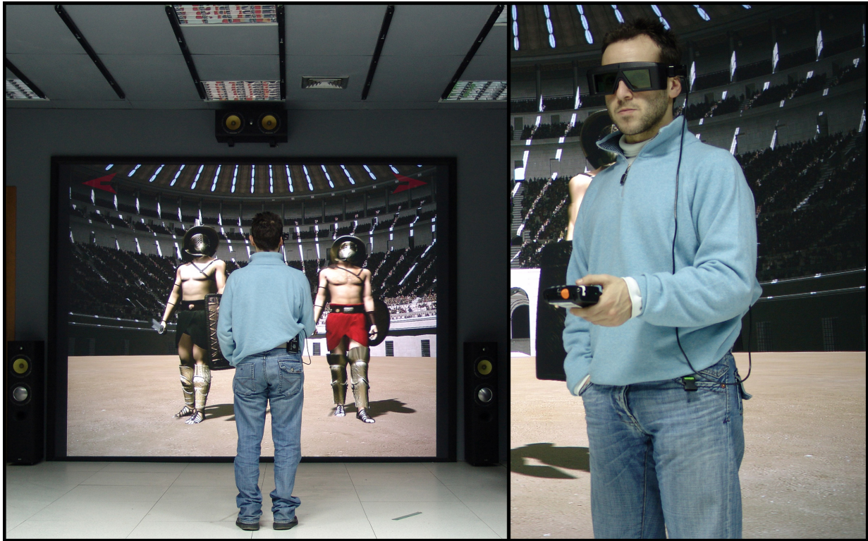
Figure 5a-5b. (a) The framework at work in the VR laboratory of DMI. The ceiling of this facility is equipped with ultrasonic based motion tracking emitter/receivers from Intersense Corp.. The retro-projection system support active stereoscopy. Navigation icons are displayed in the upper side of the screen. (b) The user wearing IR-controlled LCD Shutter Glasses, 6DOF head motion tracker (wired to a pocket wireless transmitter), and 6DOF hand motion tracker plus wireless joystick.
