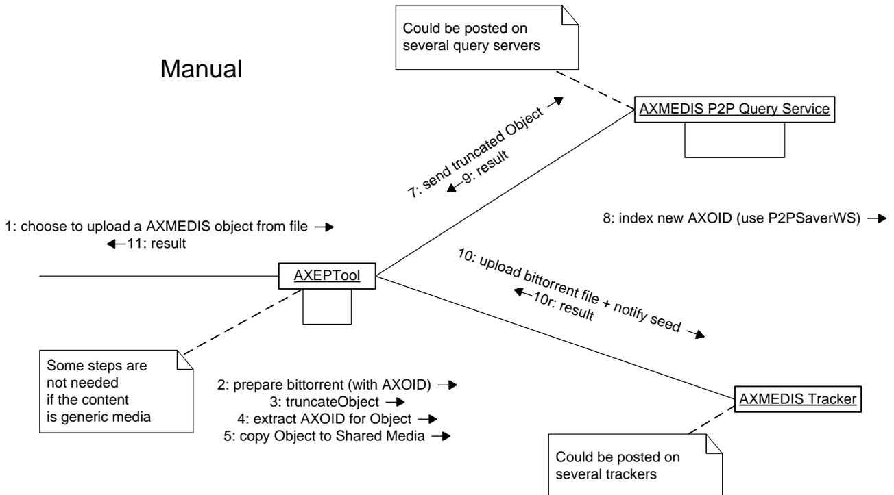
In the manual version some content manipulations which has been performed by AXCP, has to be done by AXEPTool, the AXOID has to be extracted for augmenting bittorrent, and the AXMT file (truncated object) has to be posted for future queries.
