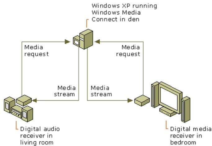
**Figure 8 – Diagram showing network devices streaming protected content**
