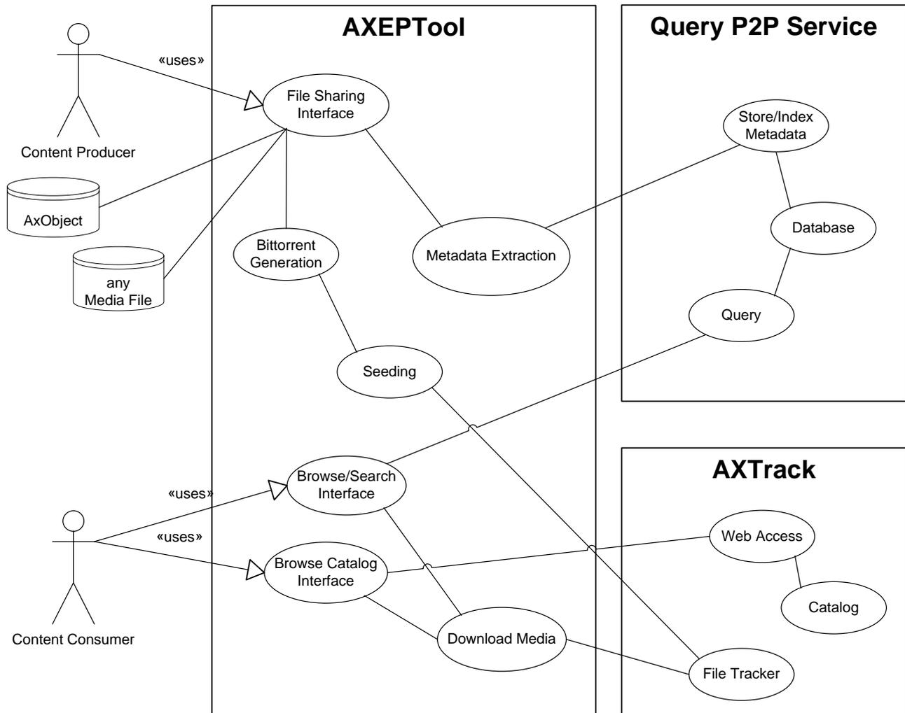
The content producer connects to a file sharing interface and use it to put the file on the peer to peer network. First metadata and bittorrent info are generated locally from the file. Those metadata are then uploaded to one or more AXMEDIS P2P Query Service, where they are indexed for subsequent query, and to one or more AXTrack Web Service as seed notification. The File Tracker starts keeping track of the files.
