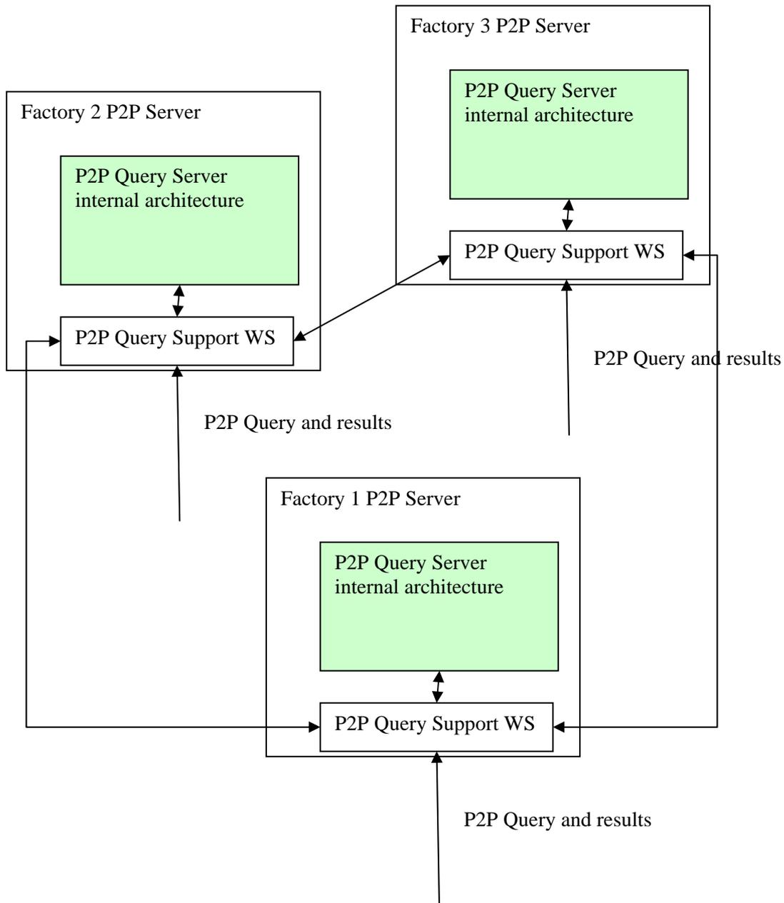
In this model the query on each factory can propagate to automatically to other factories and the results are collected together by the P2P Query Support WS layer of each factory that became then a complex component replicating the functions of the MainQuerySupport at the P2P level.
