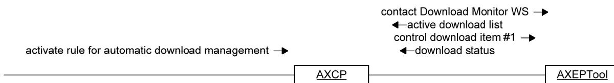
In the last diagram the AXCP is put as an intermediate in the AXEPTool control. In this case it allows the script function to operate as the user on the GUI (i.e. looking what is downloading and controlling those processes).
