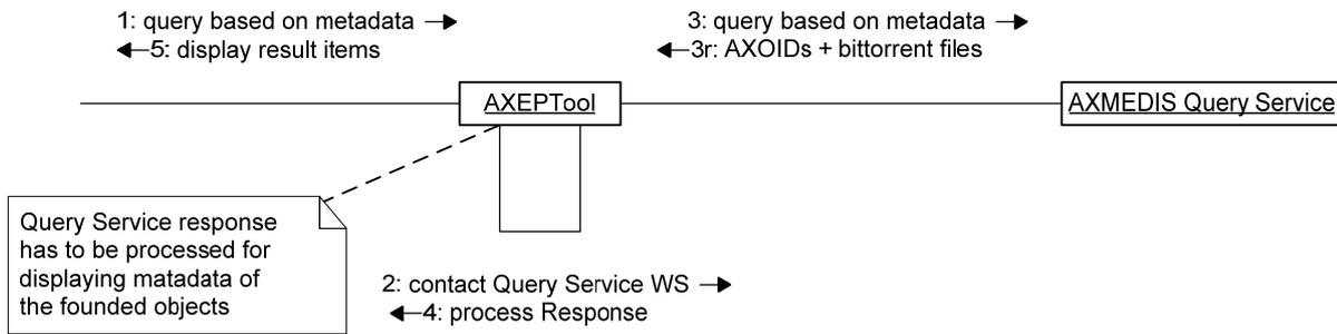
The first diagram shows the interaction between AXEPTool and AXMEDIS Query Service. The action is simply to redirect the user query to the Query Service collecting in the response information regarding the matching objects. The WS response is processed, since all the present metadata have to be attached to the query result items.
