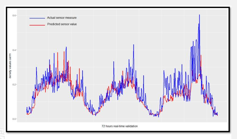
The diagram refers to one in particular of the sensors, and it displays the predicted vs actual values over the time in the 72 hours validation.
