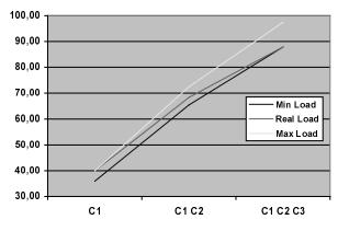
The figure reports the load of the network. In order to measure the effective performance, three couple of machines have been tested separately so to evaluate the maximun load on the HUB. The HUB has been guaranteed to have at least 90% efficiency under any workload conditions. C1, C2, C3: the three couples versus the load shown in Mbps.
