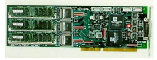
The SPARK system is based on a sinchronous multiprocessor architecture using IRIS custom-designed digital signal processing units. Each DSP board is based on three custom DSPs connected in a synchronous configuration and operating in parallel at full speed. The total aggregate computing power is 150 MIPS (peak) per board, and on-board interconnection bandwidth reaches 26 Mbit/s.
