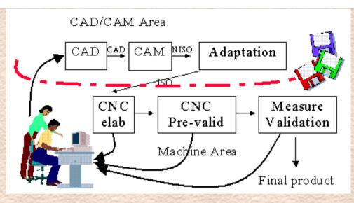
In the industries producing templates, there exists a strong interest in the integration of CAD/CAM with the factory part in which MMs, measurement systems, robots, etc., are present. The integration must be supported by a fast and reliable communication between these two areas for making available
