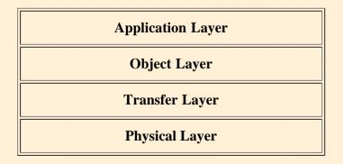
The Intel 82527 chip was chosen for our CAN module and it will realize the physical, transfer and object layer of this structure. The CAN system it is based on a packetized communication, there was four frame type:
