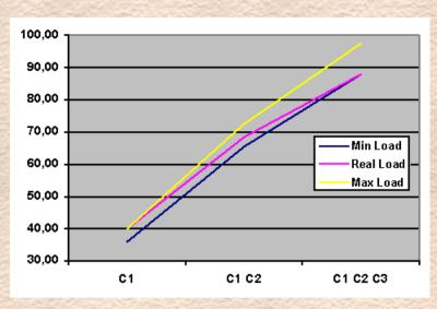
The figure reports the load of the network. In order to measure the effective performance, three couple of machines have been tested separately so to evaluate the maximum load on the HUB. The HUB has been guaranteed to have at least 90%.
