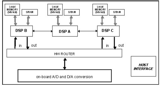
Architecture of the SPARK prototype system
