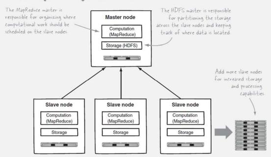
A significant advantage of using the Hadoop distributed architecture is the capability to efficiently and easily scale by adding inexpensive commodity hardware to the cluster.
